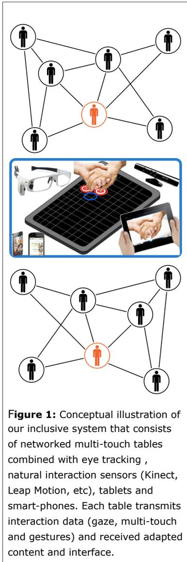
**Figure 1:** Conceptual illustration of our inclusive system that consists of networked multi-touch tables combined with eye tracking, natural interaction sensors (Kinect, Leap Motion, etc), tablets and smart-phones. Each table transmits interaction data (gaze, multi-touch and gestures) and received adapted content and interface.
